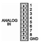
Figure 3-8: Analog In Connector
